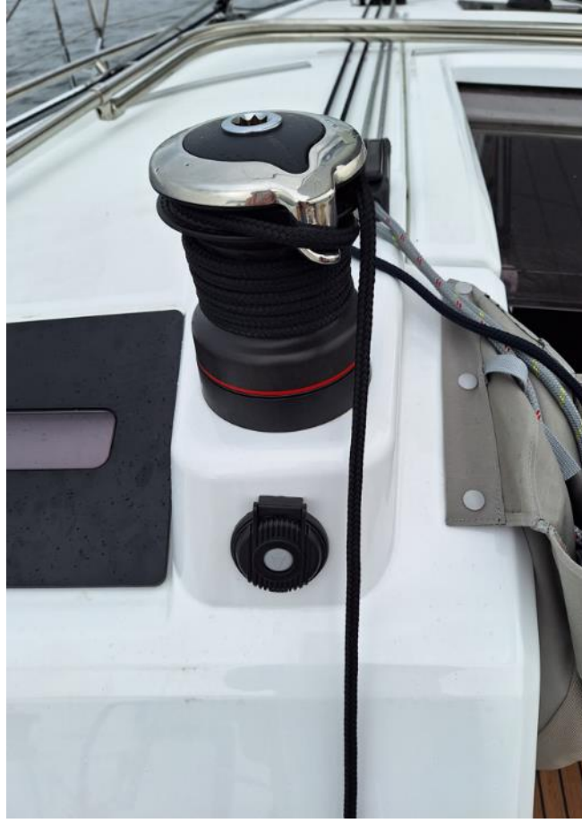
Electric winch on the port side
